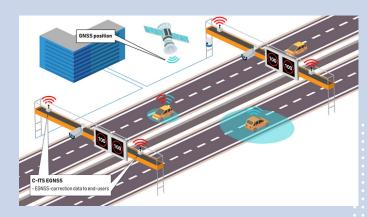
Routing recommendations within and between lanes based on the road wear map, provided via C-ITS messages
