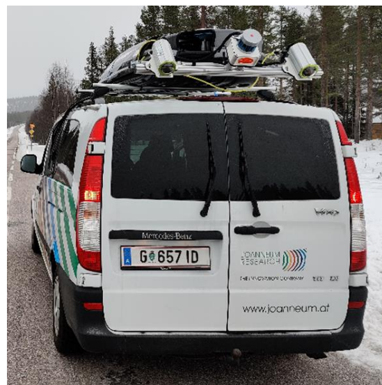
Figure 23: The road wear sensor system in Finland with the actual ESRIUM sensors (mainly the two high-resolution cameras).
