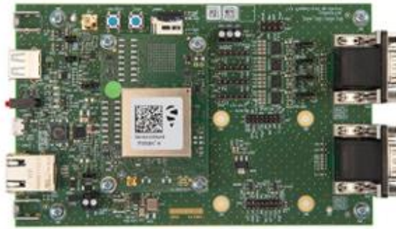
Figure 15: Septentrio mosaic-H EGNSS Development Kit to be used during preliminary tests for the localization of the automated driving demonstrator vehicle.
