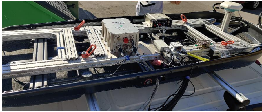
Figure 22: Detailed view inside the roof box with the reference GNSS/IMU system for evaluation in the centre and the GNSS unit. The actual optical road wear sensor components for ESRIUM (cameras and LiDAR) are mounted on the back.
