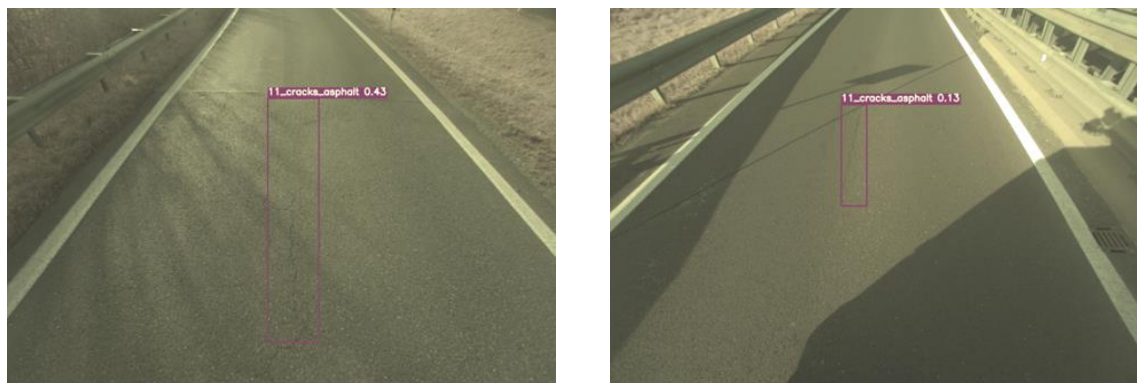
Figure 30: Detection results with YOLOv4 detector trained on ESRIUM data on new unseen data.
